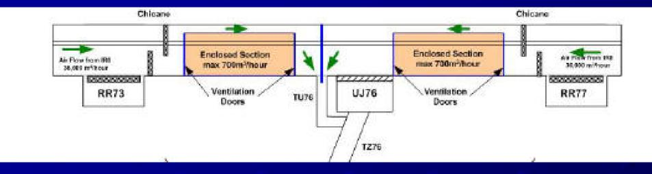
The collimators will be enclosed - ventilation doors - collimators between D3 and D4 should NOT be there for the test. See below.
